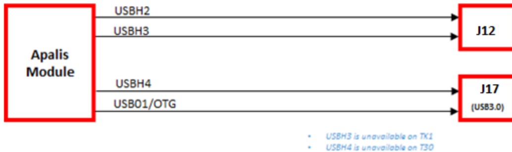
Figure 3 USB Signal connection for Eaglet baseboard
